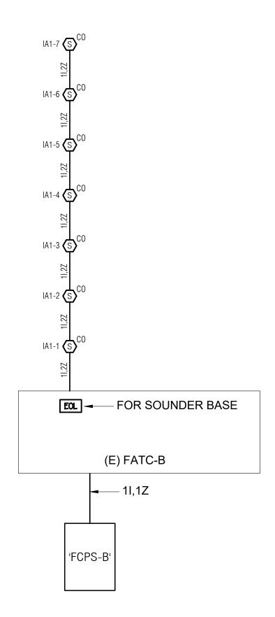
NOTE: ALL WIRING TO BE IN RACEWAY
