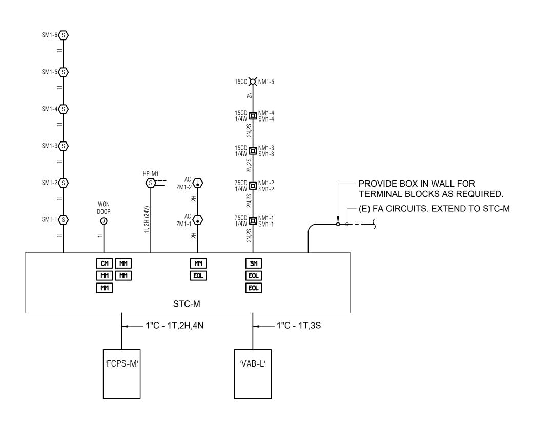
NOTE: ALL WIRING TO BE IN RACEWAY
