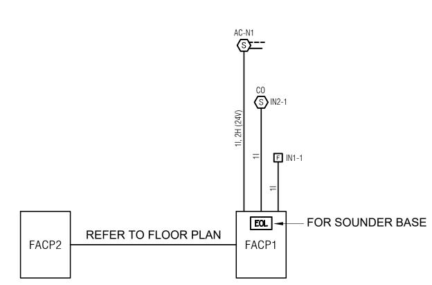
NOTE: ALL WIRING TO BE IN RACEWAY
